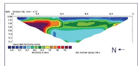
Fig. 10 Vertical section obtained by depth profiling at the southern edge of the tell.
