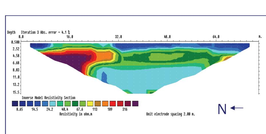
Fig. 10 Vertical section obtained by depth profiling at the southern edge of the tell.
