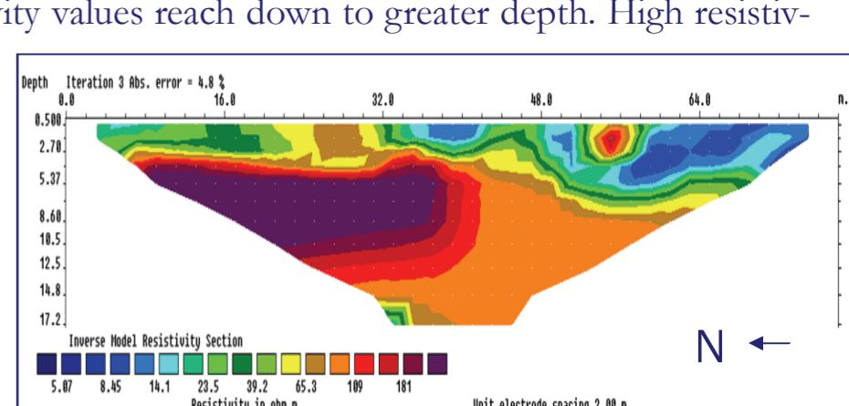
Fig. 9 Vertical section obtained by depth profiling at the centre of the tell.
