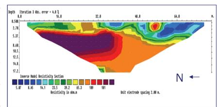
Fig. 9 Vertical section obtained by depth profiling at the centre of the tell.
