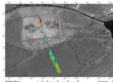
Fig. 7 Positions of geoelectric depth sections.
