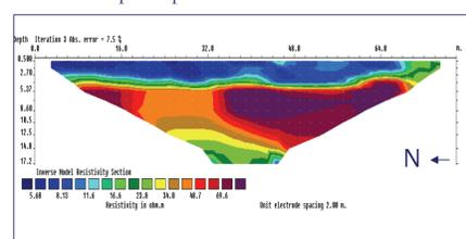
Fig. 8 Vertical section from depth profiling in the eastern part of the tell.
